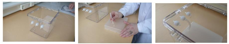
4: Do the same with the other clamps on the other holes. 5: Put the silicon tube on the inner chamber and put it in the bottom of the outer container.
