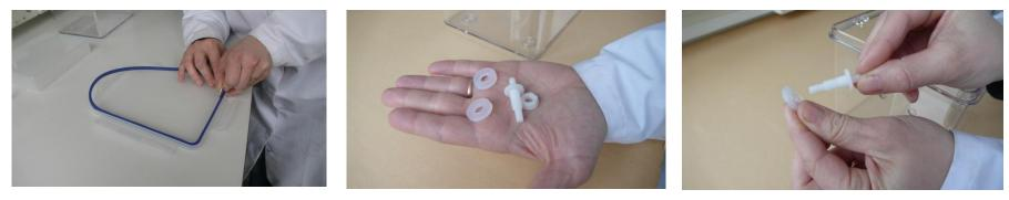
1: Put the blue silicon ring in the lid. Press down careful with a coin. 2: Put one silicon ring on the clamp.
