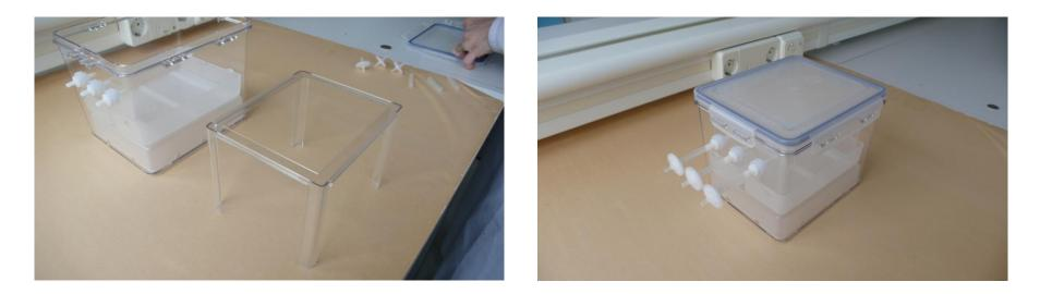
7: Put the frame with the four legs above the basket and then close the container with the lid.
